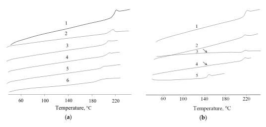
**Figure 4.** Differential scanning calorimetry (DSC) curves of blends PEI/OPSU (**a**): 1—PEI; 2-5—PEI+10, 15, 20, 30% OPSU, respectively; 6—OPSU and PEI/PC (**b**): 1—PEI; 2-4—PEI+10, 15, 20% PC, respectively; 5—PC.
