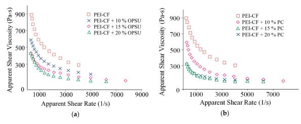
Figure 7. Dependence of the PEI-CF melt viscosity on the content of OPSU (a) and PC (b).
