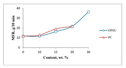
**Figure 2.** Dependence of melt flow rate polyetherimide (MFR PEI) on the content of oligophenylene sulfone (OPSU) and polycarbonate (PC).
