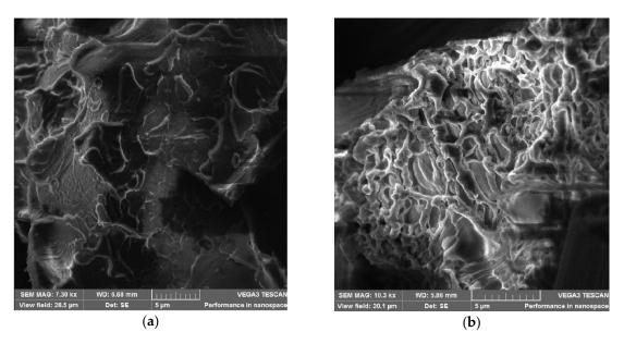
**Figure 9.** SEM images of the polymer matrix of carbon-filled samples: (a)—PEI-CF + 15% OPSU; (b)—PEI-CF + 10% PC.
