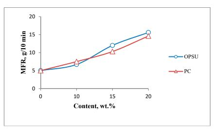
Figure 6. MFR PEI-carbon fibers (CF) with different content of OPSU and PC.
