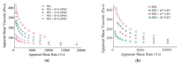
Figure 3. The dependence of the PEI melt viscosity on the content of OPSU (a) and PC (b).
